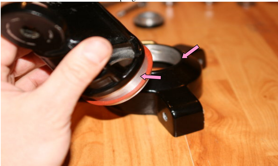
Pic # 5 - Pink arrows indicate where I put grease
