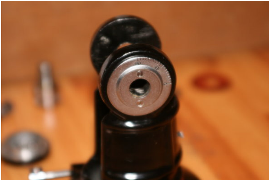
Pic #6 – Notice the screws that hold the Latitude Indicator Circle. Nice feature.
