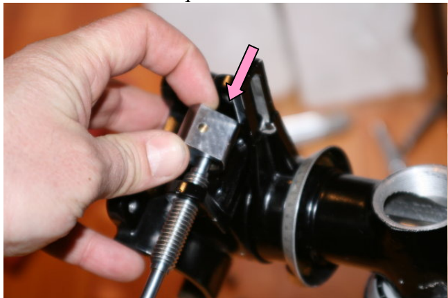
Pic #30 – Hold square nut and thread
