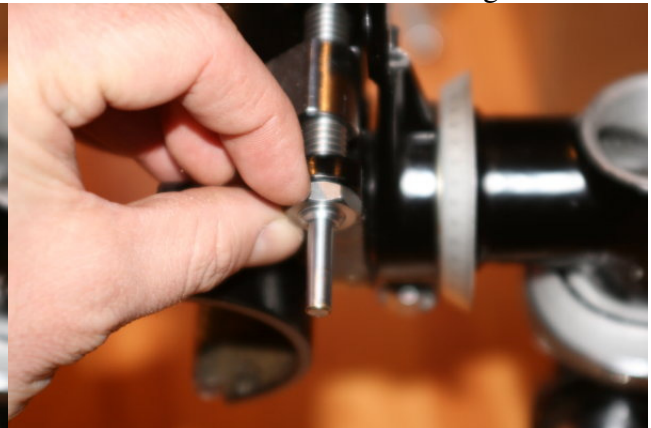
Pic #33 – Thread locking nut
